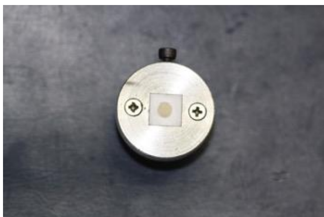
Figure 3. Test specimen in the shear test device. Source: Own authorship.
