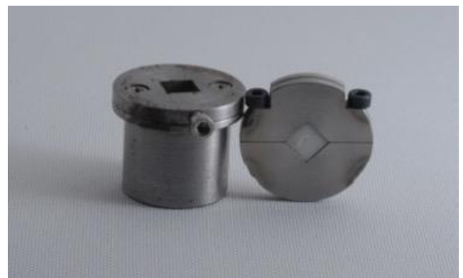
Figure 1. Device used in the shear test and matrix to accommodate zirconia. Source: Own authorship.
