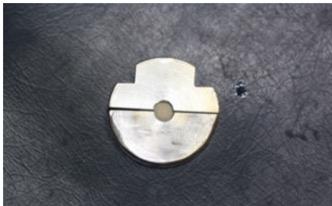
Figure 2. Metal matrix where coating ceramic is applied. Source: Own authorship.
