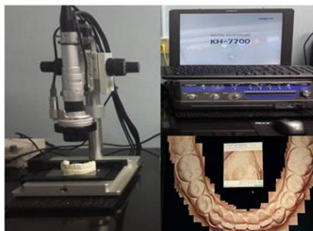
**Figure 1.** Fabrication of the digital models via Hirox digital stereomicroscope
