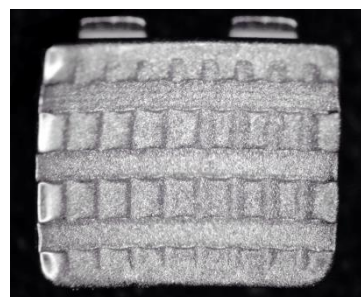
Figure 2. Surface of the Mini Dyna Lock™ bracket base seen with a stereomicroscope (magnification, 10×).
