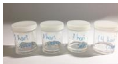
Figure 6. the stainless steel Wire immersed in artificial saliva.
