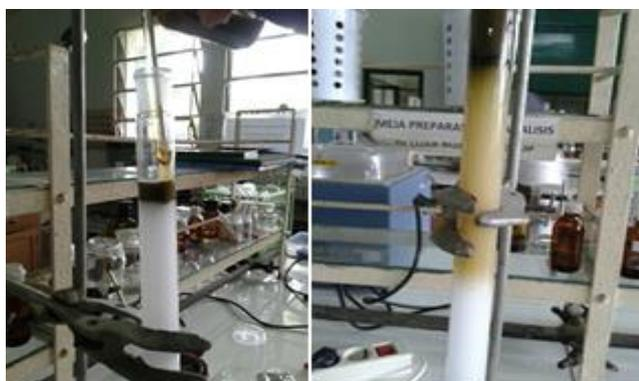
Figure 4. Chromatographic process.
