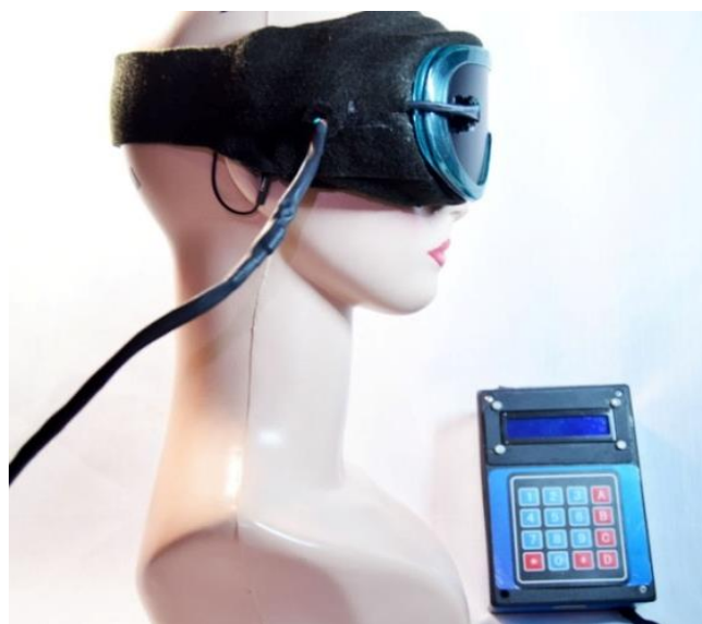
Figure 4. LED and Binaural Beats Mask prototype.
