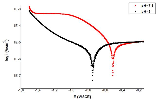
**Figure 4.** Polarization Curves of Ni-Ti after an Hour Immersion in Artificial Saliva at pH 3 and 7.8
