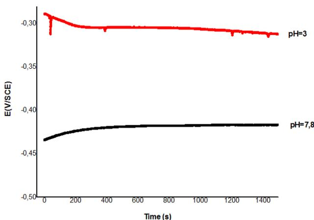
**Figure 3.** Evolution of the Open Potential of Ni-Ti with Immersion Time in Studied Solutions.
