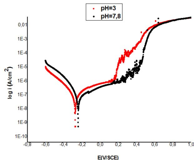
**Figure 8.** Polarization Curves of Stainless Steel After an Hour Immersion in Artificial Saliva at pH 3 and 7.8.
