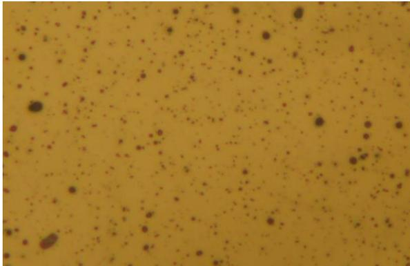
**Figure 2.** Microstructural Examination of the Investigated Ni-Ti Wire (a) under a Magnification of 300x (2)
