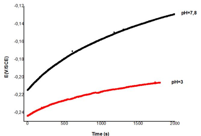
**Figure 6.** Evolution of the Open Potential for Stainless Steel an Hour Immersion in Artificial Saliva at pH=3 And 7.8.
