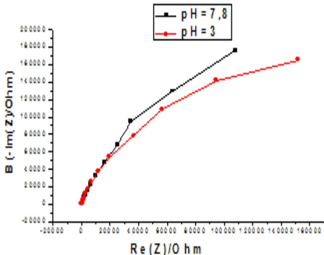
**Figure 7.** Impedance Diagram of the Stainless Steel Wire after an Hour Immersion in Different pH.
