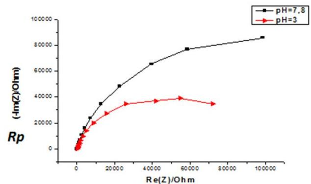
**Figure 5.** Impedance Diagram of the Ti-Ni Wire after an Hour Immersion in Different pH.
