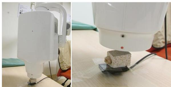
**Figure 3.** Setting of Equipment for Periapical Radiograph of the Samples.
