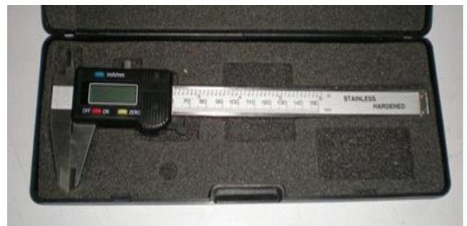
**Figure 3.** Digital caliper with a precision of 0.01 mm.
