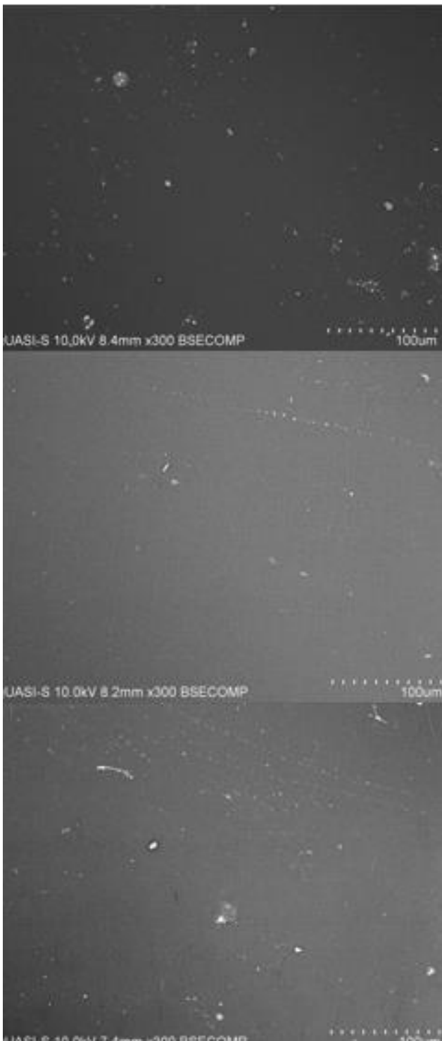
Figure 1. Initial micrograph SEM images of samples prior to mechanical brushing.
