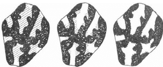
Figure 3. The activation process of carbon gradually during the treatment temperature. Source: International Journal of ChemTec Research-Activated Charcoal 8
