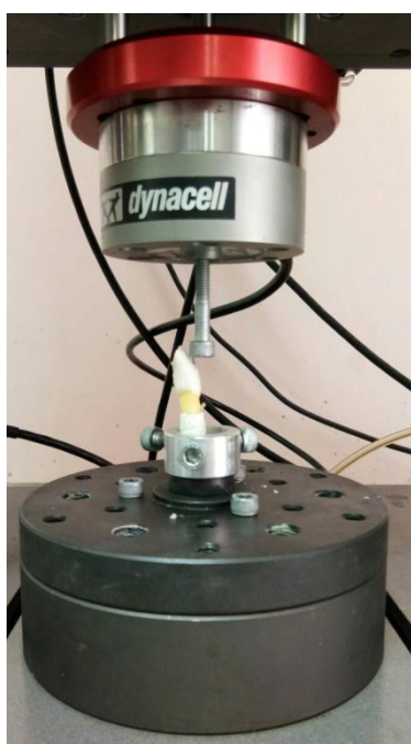
Figure 5. The bonding strength tested using Instron Universal Testing Machine
