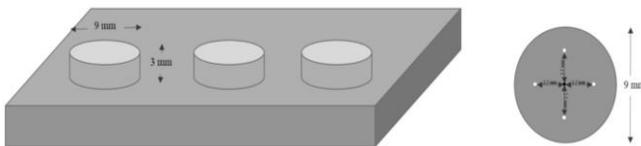
**Figure 1.** Diagram showing silicone mold for cylinder-shape specimen and measurement points for microhardness test.
