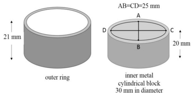
**Figure 3.** Diagram showing stainless steel mold for disc-shaped specimen and measurement points for dimensional change.
