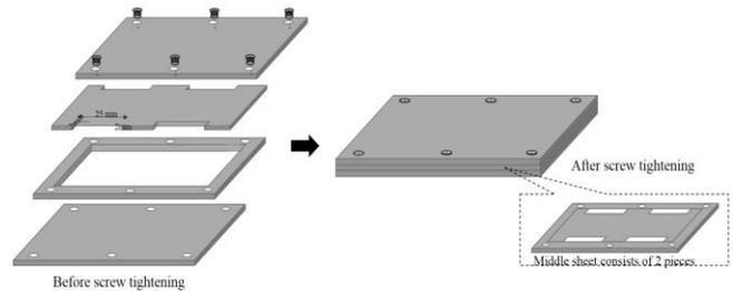
**Figure 2.** Diagram showing stainless steel mold for bar-shape specimen for flexural strength test.
