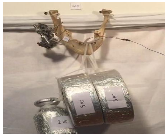
Figure 4. Carrying out tests of the load on the structure of the "EXOCHHEL" apparatus.
