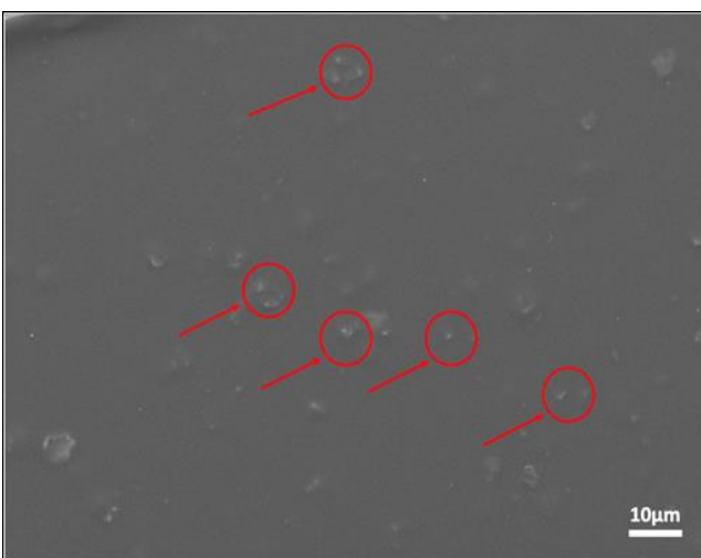
Figure 6. SEM result sample varnish with \text{CO}_3\text{Ap} and \alpha\text{-TCP} (4 smears).
