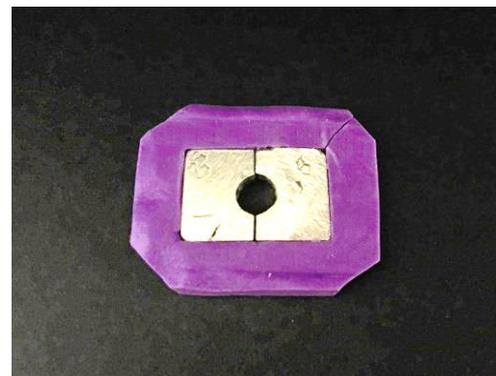
**Figure 2.** The metal mold (5 mm in diameter X 2 mm in thickness) used in the study.
