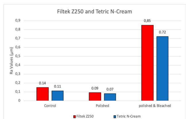
**Figure 3.** Mean surface roughness (Ra) values in  $\mu\text{m}$  of the six subgroups being tested in this study.
