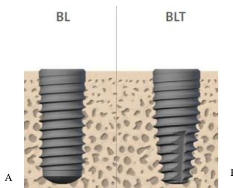
**Figure 1.** Implant thread designs. **A.** BL: bone level. **B.** BLT: bone-level tapered<sup>27</sup>
