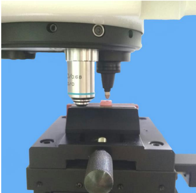
Figure 2. Surface hardness test.
