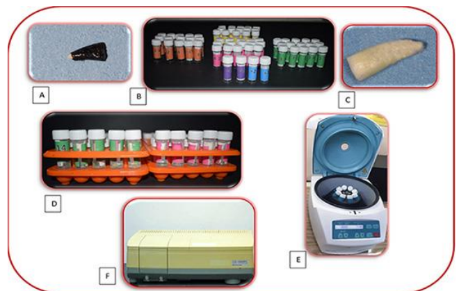
Figure 1. A. Root coated with two layers of nail varnish with the exception of apical 0.5 mm, B. The samples dipped for 24 h at 37°C in a neutralized buffer 2% methylene blue solution, C. Varnish removed using BP blade and polishing disks, D. Samples in a plastic container containing 4 ml of 65% nitric acid for 3 days, E. Centrifugation of this solution done at 4000 rpm for 7 min, F. Spectrophotometer device for reading the optical density of the dye that penetrate samples.
