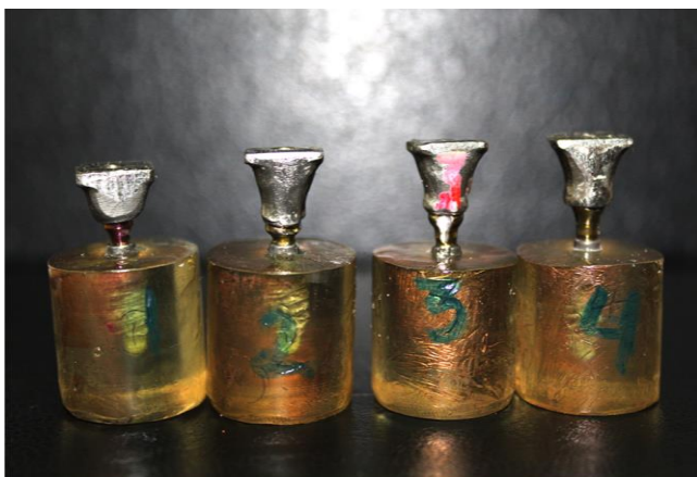
Figure 1. The metal tubes attached to the four abutments.
