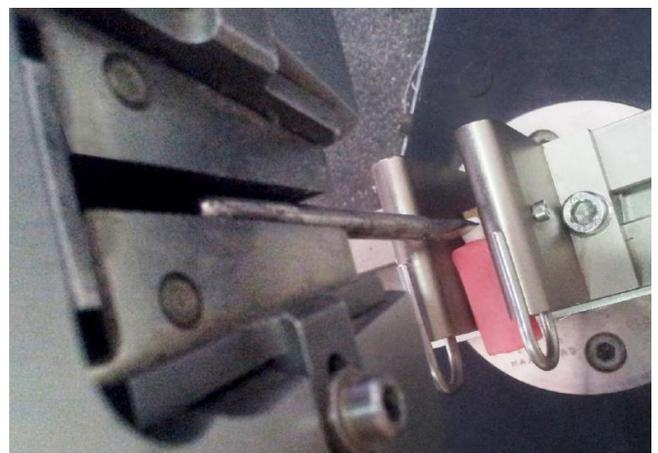
**Figure 7.** Load applied on sample mounted on Instron.
