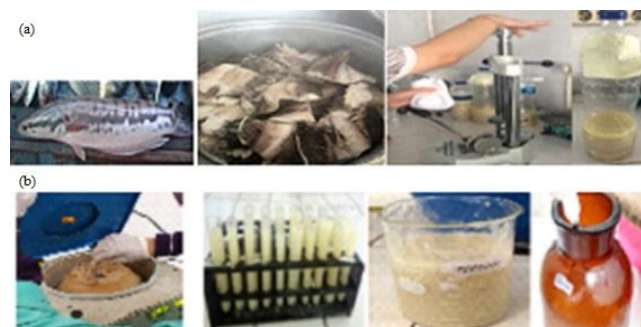
Figure 1. Preparation of Toman fish extract, where the meat of Toman fish was boiled and pressed using a hydraulic press (a) and the centrifuged supernatant was kept in the dark glass bottles (b) for further use.
