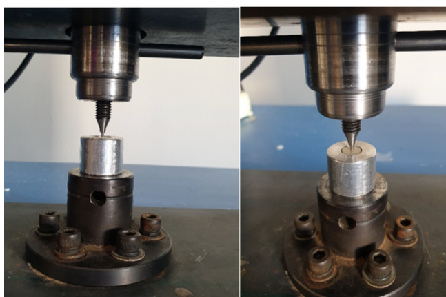
Figure 3. Disc specimen under loading showing specimens in contact with the piston using Jinan Testing machine.
