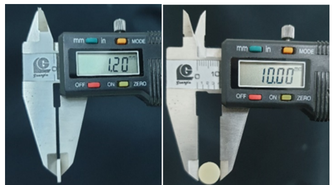
Figure 2. Guanglu digital caliper used to check dimensional accuracy.
