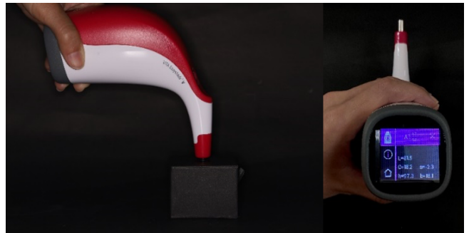
Figure 3. L*a*b values measurement using Vita Easyshade V.
