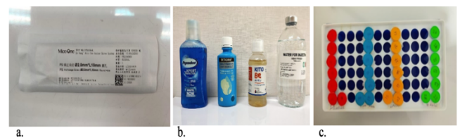
Figure 1. (a) Stainless Steel TAD, (b) Four groups of mouthwashes, (c) SS TAD samples immersed in four mouthwash groups.
