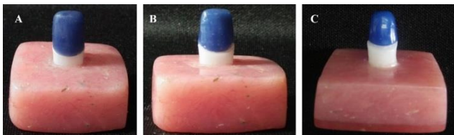
Figure 2. Wax-Up Coping Photographic Images, (A) inlay wax was placed exactly in the area of labio marginal (0.3 mm), (B) inlay wax was positioned only at the edge of surface area of labio marginal (0.3 mm), (C) inlay wax on 1.5 mm of surface area of labio marginal .
