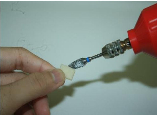
Figure 11. The sample was trimmed by using straight handpiece tungsten carbide bur.
