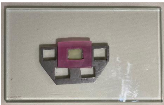
Figure 2. The modelling wax with 1 mm thickness was used to standardize the distant between the light cure and sample.
